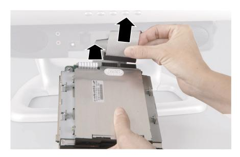
**5** Connect the drive cables to the drive adapter card on the new drive pack. The drive cables and connectors are "keyed," which means that they can only be plugged in one way.
